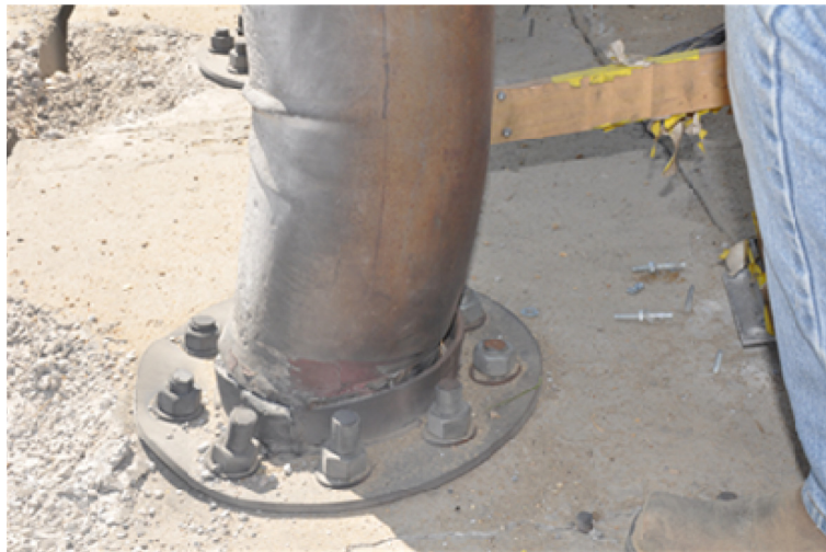
Fig. 9. Damage to Rulon tape and slip of Specimen MSJC1 over collar
