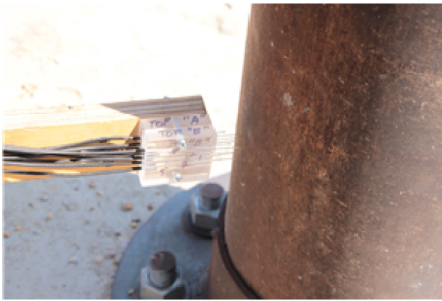
Fig. 19. Shorting pin assembly on back of MSJC2 (Block A is hidden behind Block B)
