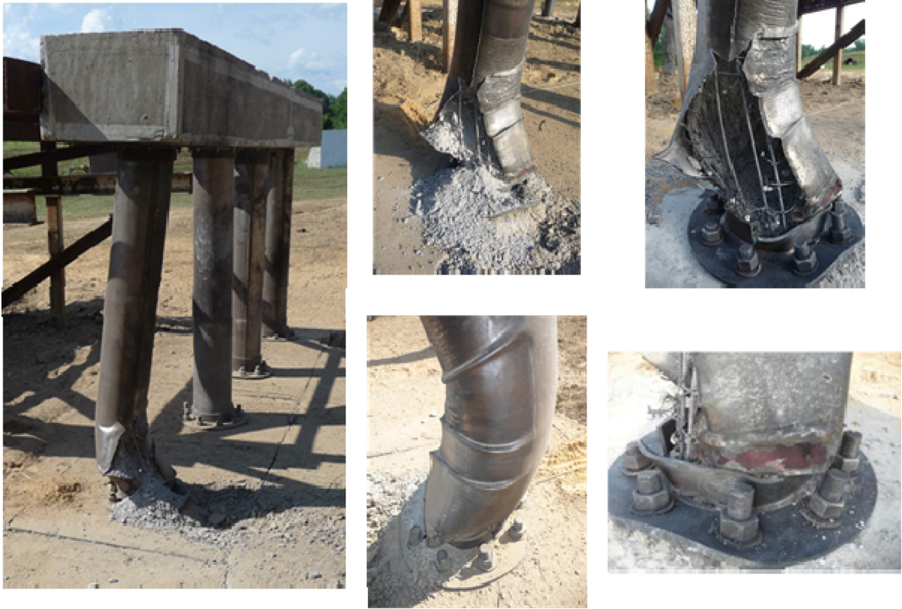
Fig. 18. Global view and close-up of base of Specimen MSJC4 after test
