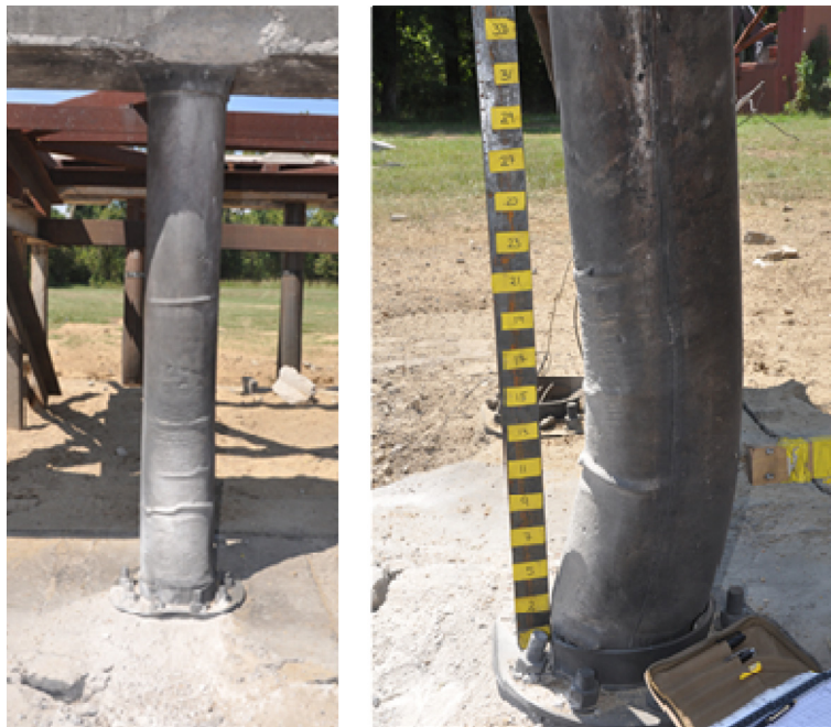
Fig. 15. Deformation of Specimen MSJC3 after second test
