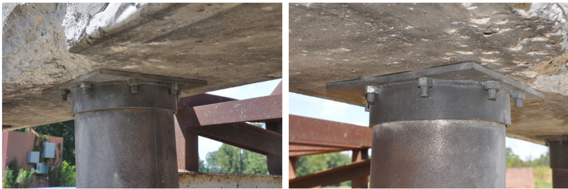
Fig. 17. State of top collar after second test of MSJC3
